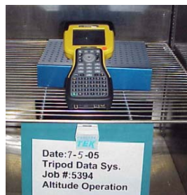
Figure 2—MIL-STD-810F Method 500.4 low-pressure test
