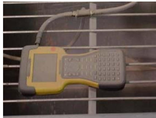
Figure 3—MIL-STD-810F Method 510.4 sand and dust test
