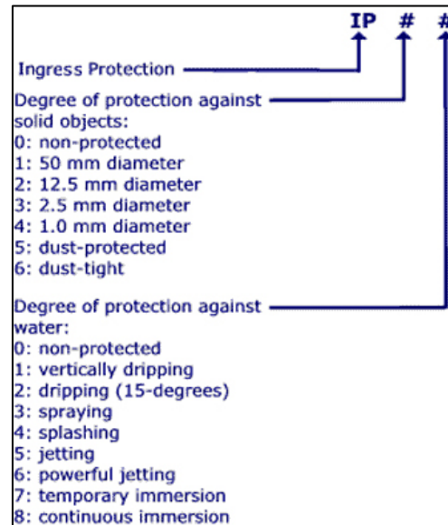
Figure 1—Ingress Protection (IP) Code definitions
